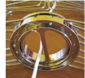
frame wires are pivoted into slots in the hub
